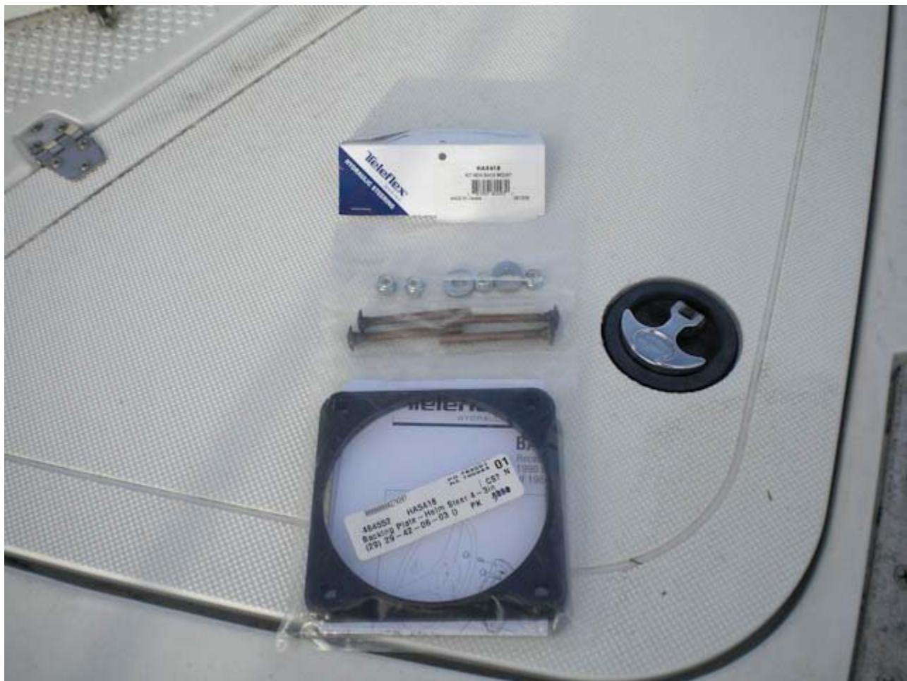
The kit comes with a paper template but the backing plate that goes inside the console is just as easy to use. I bolted it on the outside and marked and drilled the 8 holes.
