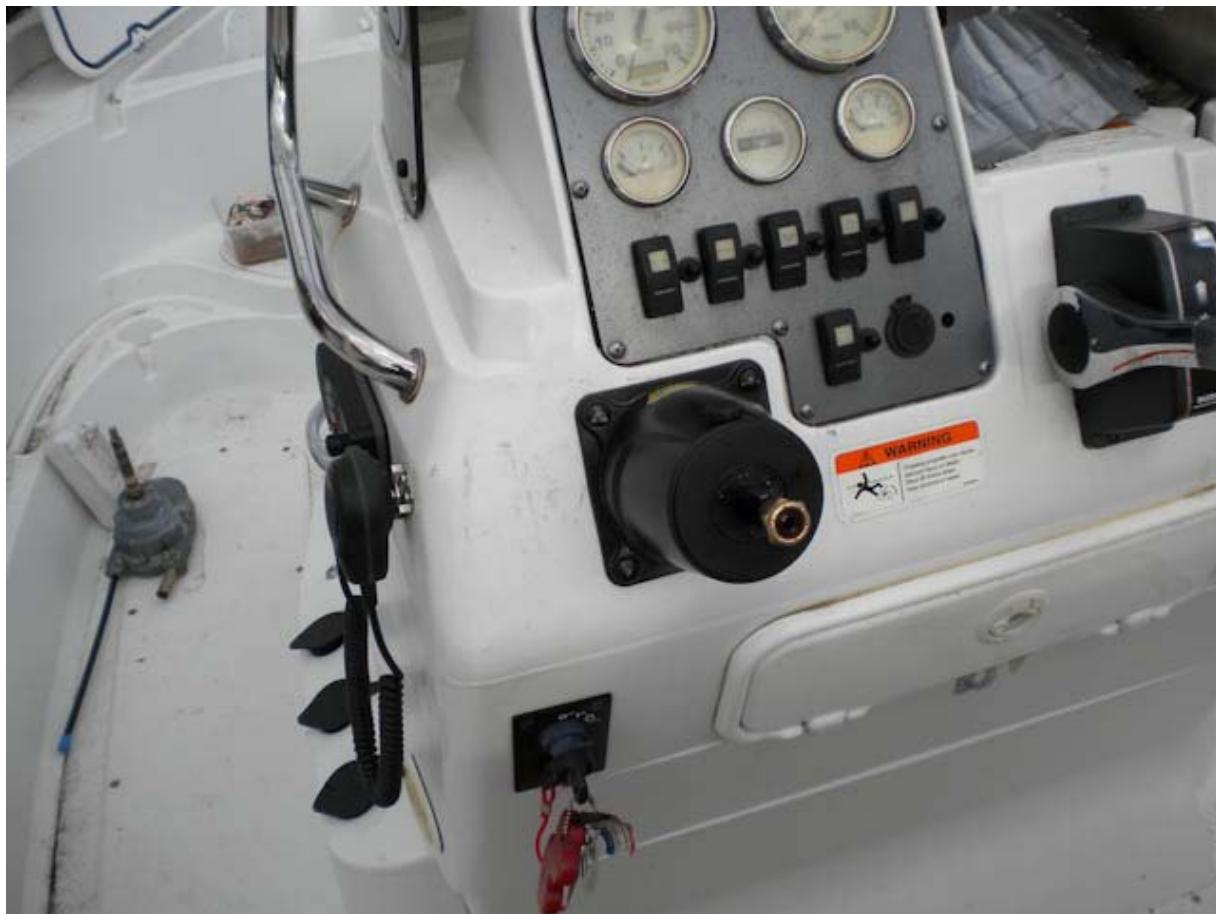
Prepare the cylinder for the outboard. In my case (Suzuki DF-140), I needed to flip the pivot plate around. Remove the 2 Hex head bolts and turn the plate around 180°.
