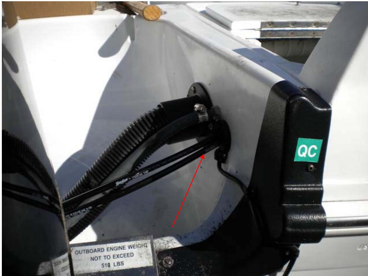
Onto the helm. First you'll need your spacer kit. The new helm pump requires a 3" hole and my old steering unit used a 3.25" hole. That didn't leave enough material for the mounting bolts. Teleflex makes a mounting kit just for that.
