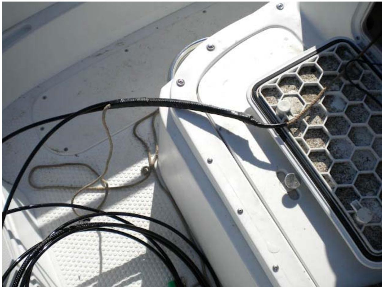
Instead, I taped one hose to the middle of the rope and pulled it through. You are pulling on the rope from the rear (stern) of the boat and feeding the hose into the conduit inside the console. You and your helper should work slow and be careful not to damage any wires.
