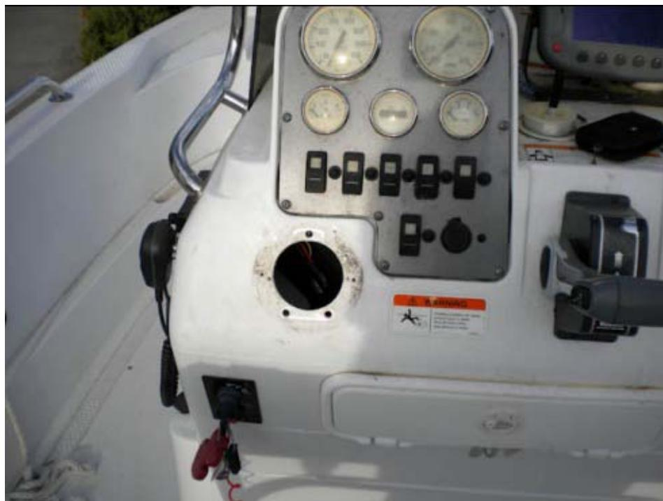
While standing at the console, pull the cable and the pull rope back through the conduit and into the console. Go slow and have your helper guide the rope through the conduit. Be careful not to damage any wires at the stern or inside the console. You will have the steering box and the steering cable come out all in one piece. Once it is removed you can undo the electrical tape and throw the steering box and cable overboard (it made me feel better).
