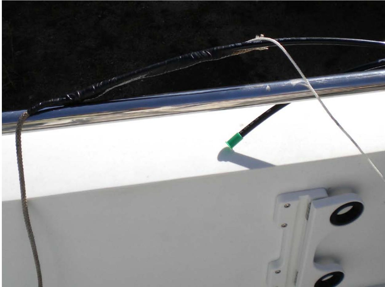
Now feed the 2 hoses into the splash well. In my case, they fit inside the fitting that supported the original steering cable.
