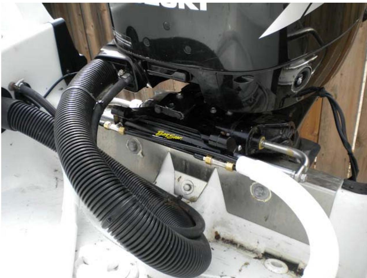
Fill the Helm pump with fluid (provided in the kit) and bleed the system as described in the instructions. Check to make sure everything is working and the motor is turning in the right direction.
