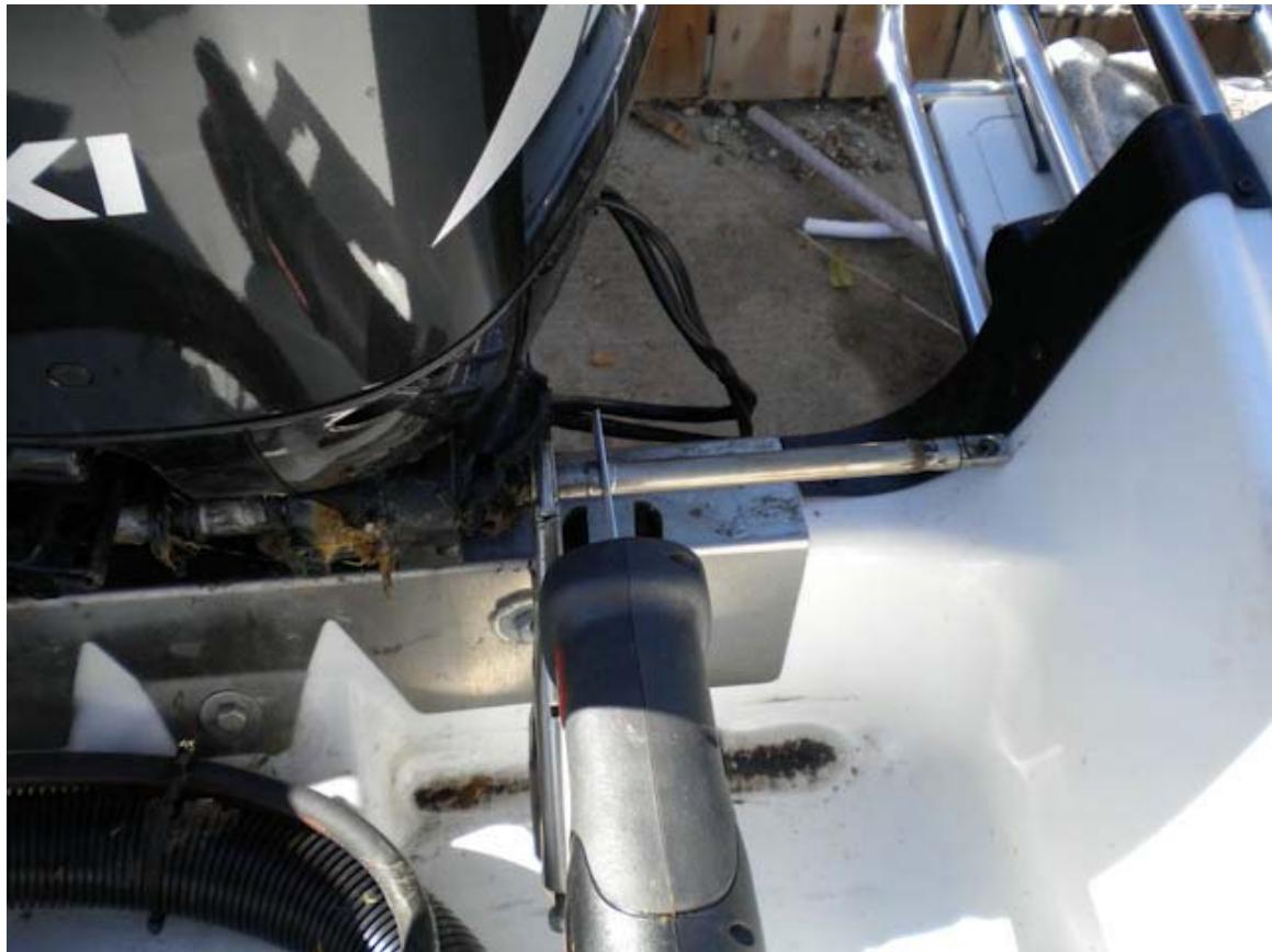
I made the cut, pulled the remaining piece through with the vise grips and it came out. Once I backed off the nut (on the other side) I had 3 short pieces. The next step is to remove the cable.
