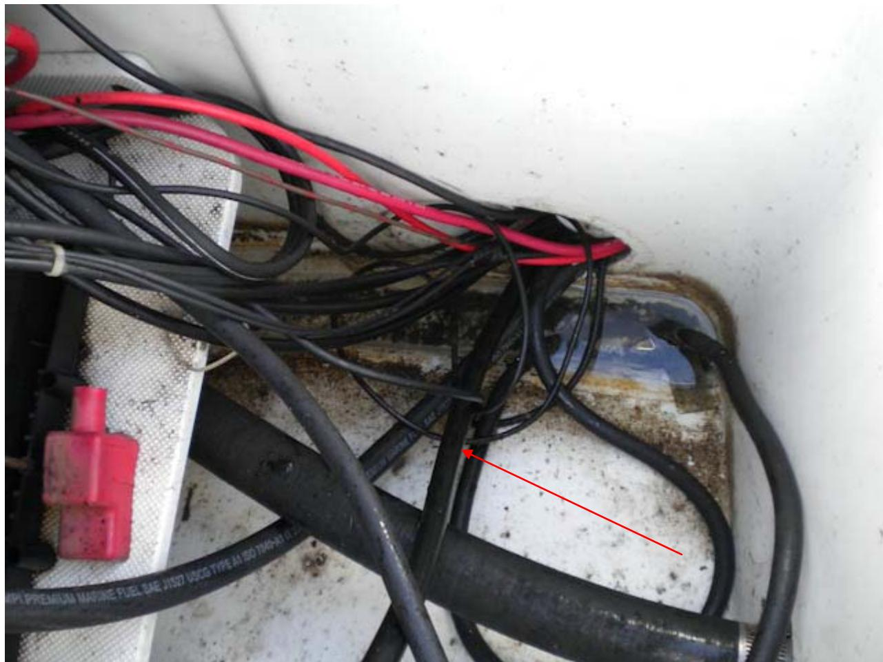
On my boat, it was easier to pull the cable back through from the console end. I taped a pull rope on the end of the cable. Overlap the rope and the cable for about 10"-12" and use plenty of tape. I made sure I had at least 50 feet of rope for a boat my size.
