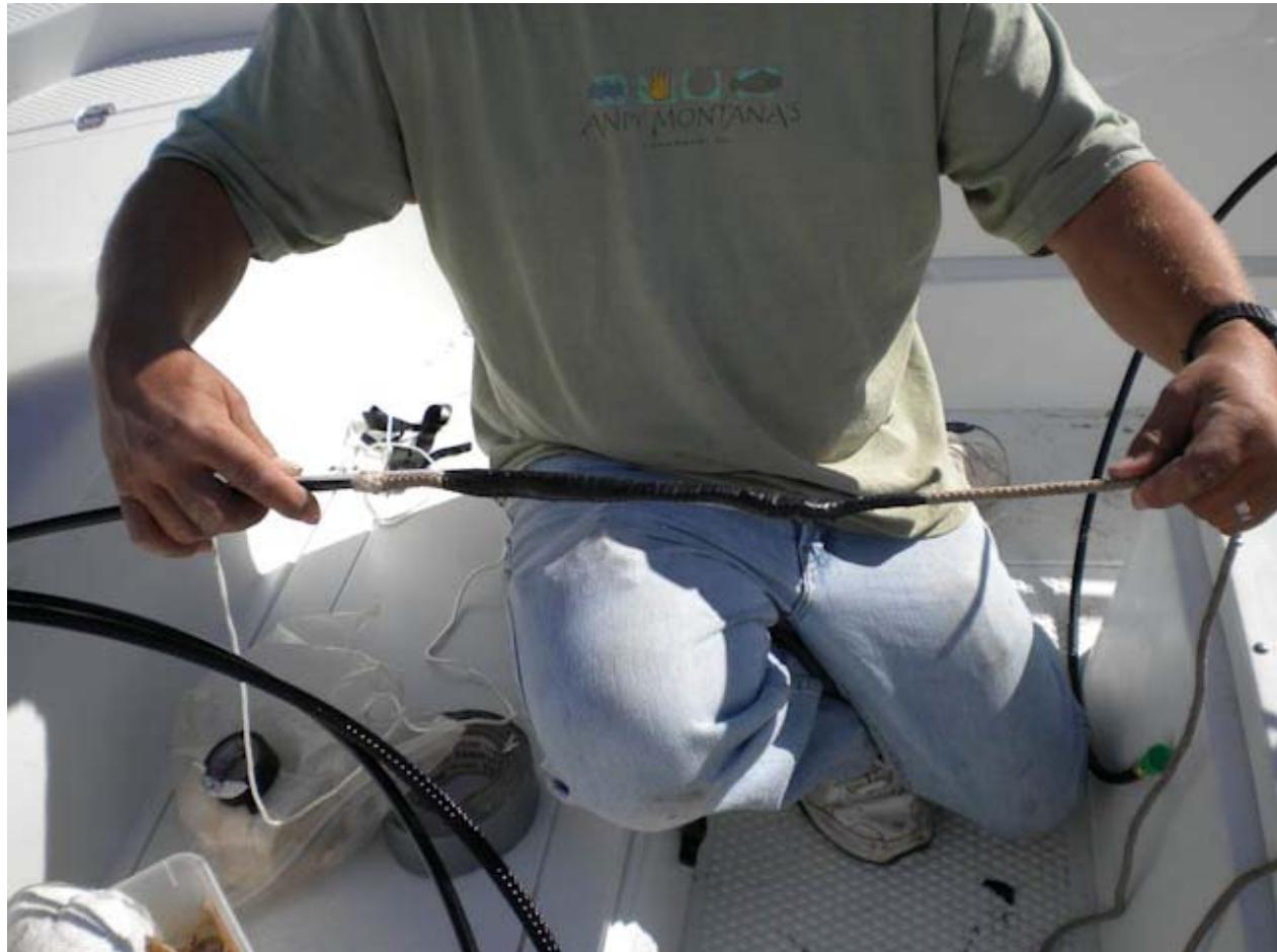
If you did it right, it will look like this. This is a picture from the rear (stern) of the boat. The green plastic end is from the first hose. The red plastic end is under the tape and you can see the extra cord I pulled for future projects. I removed the tape and wound up the cord and stored it under the seat. The rope I'll save for something else.
