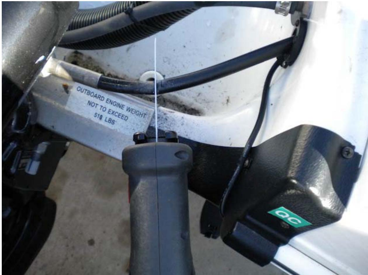
Next, I cut the other side of the cable. I used vice grips to hold it in place and keep it from spinning.
